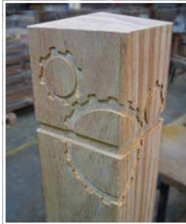
Cogwheel wrap-around design, shown fresh from the CNC, and with painted infill.
