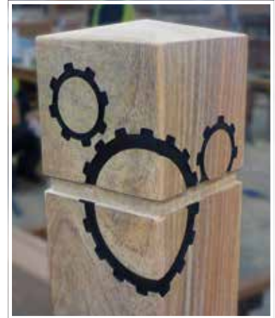
Cogwheel wrap-around design, shown fresh from the CNC, and with painted infill.
