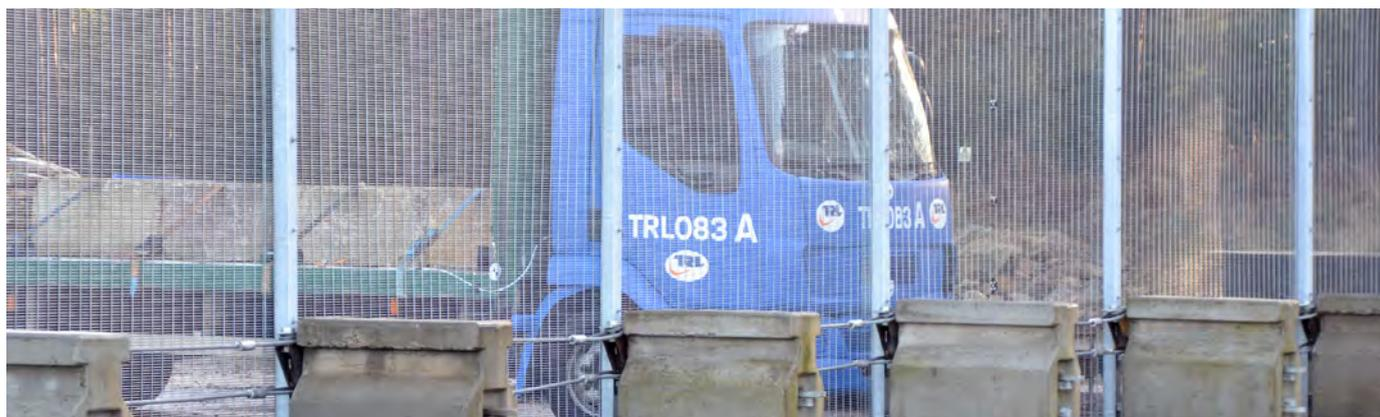
BSi PAS 68 is the a Publicly Available Specification for vehicle security barriers and fences. It has become the standard and security benchmark for Hostile Vehicle Mitigation (HVM) equipment and is the specification against which the perimeter security equipment is tested to prevent vehicle borne attacks.
