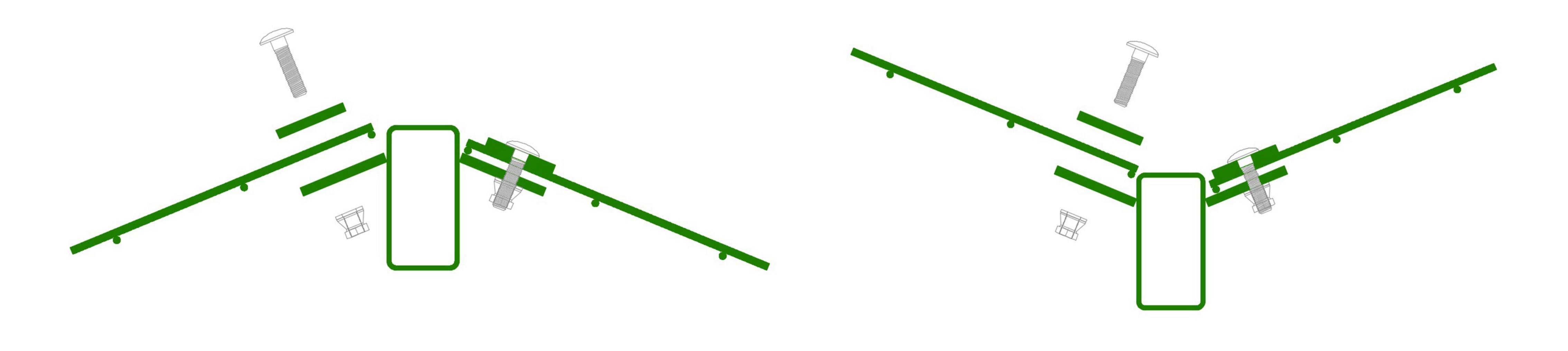
MAX change of direction is 45°. A flange is welded at the post at 45°, or a post with two welded flanges at 22.5°
