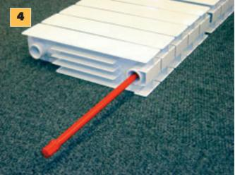
Rotate the nipple using the nipple key, so that it pulls the 2 sections together. At this stage only rotate the nipple by one turn. Repeat with the other nipple.Repeat the above, alternating so that both sections are pulled gradually together and ensuring they are kept parallel.
