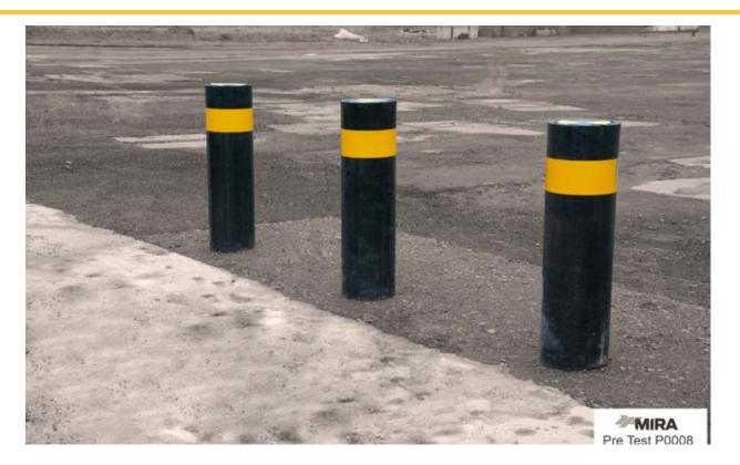
**The Avon Resilience SSF100 Bollard** is a super shallow foundation bollard, designed to provide stand-off hostile vehicle protection for infrastructure without the need for deep foundations.
