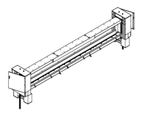
Barrier Lift System with electro-hydraulic drive in separate drive cabinet, guide Design:
