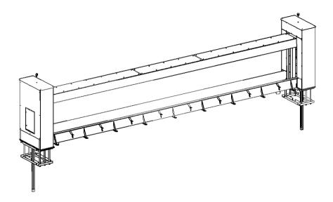
**Design:** Barrier Lift System with electro-hydraulic drive in separate drive cabinet, guide
