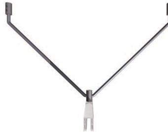
When no suitable wall fixing is available, V-Hanger is used instead of Rod Suspender to prevent lateral sway. Fixed to the track and to the ceiling via Ceiling/Track Bosses.
