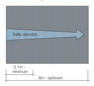
To comply with BS 7953 a minimum traffic direction of 2.1m would be required, however many experts recognise that 6 metres (or 8 to 10 foot falls) is the optimum walk-off length of entrance matting, which would allow for effective dirt and moisture removal, thereby preventing floors becoming dangerously slippery.
