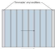
Compress mat towards the endfiller to remove any slack **before** trimming endfiller at other end of mat
