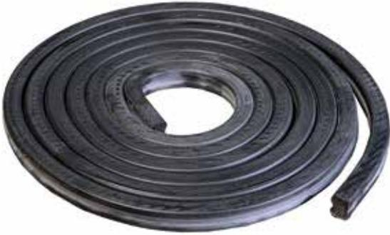
Koster Quellband is used as a waterstop in concrete construction joints. The robust strip is simply nailed onto an existing joint face before the consequent concrete pour. Any leakage through the joint activates the Quellband.
