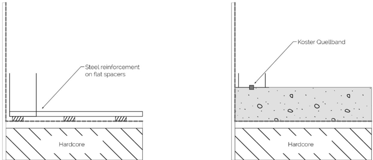
Koster Quellband should be included in the applicable slab construction joints.
