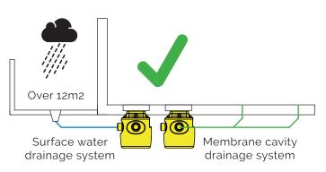
Pump stations for a cavity system & external area MORE THAN 12m2
