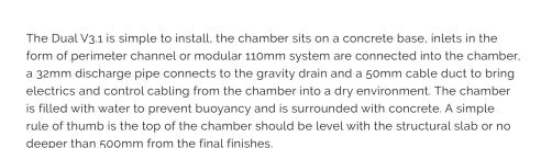
The installation is to be topped off with a double sealed cover supplied by the contractor to tie in with the general floor finish. Remember this product need to be accessed for service so care should be taken with its location.
