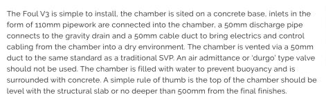
The whole lot is topped off with a double sealed cover supplied by the contractor to tie in with the general floor finish. Remember this product need to be accessed for service so care should be taken with its location.
