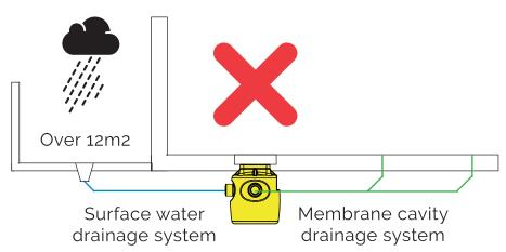
Pump station for a cavity system & external area MORE THAN 12m2
