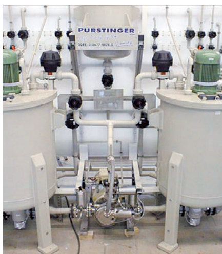
Slurry supply (Pürstinger company)
