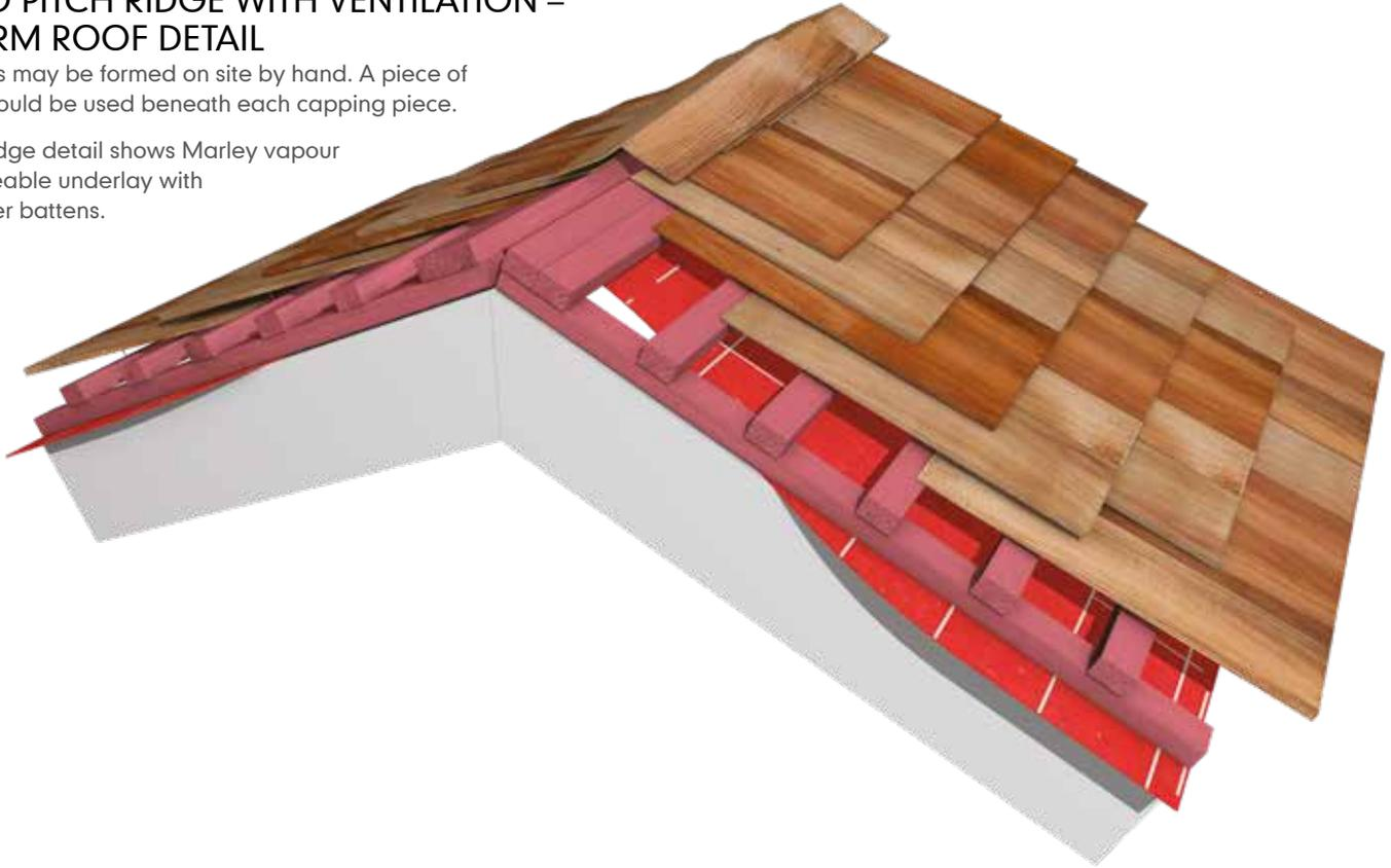
Ridge cap manufactured on site using 190mm and 200mm shakes. Each shake is chamfered and fixed with an alternate overlap
