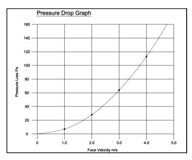
The above graph enables the predicted pressure loss, or resistance of the louvre to be obtained at various airflow rates.
