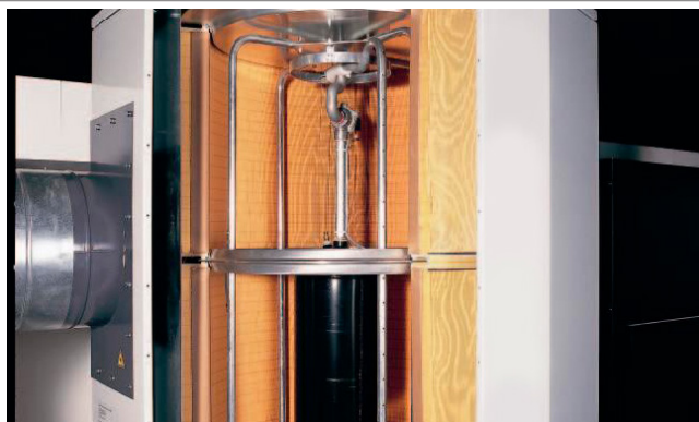
RoboCleanPlus filter cleaning system that arranges automatic sectionwise cleaning of the filter cartridges by compressed air
