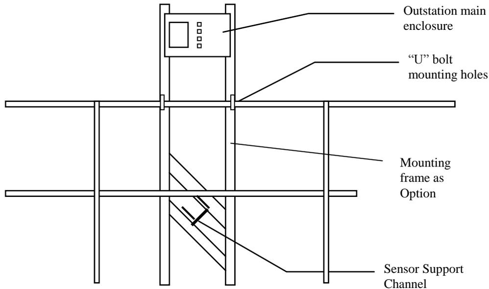
When mounted the display should be visible from the walkway and usually between waist and shoulder height.
