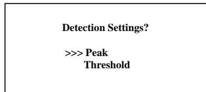
Select the required echo detection algorithm required then press the **Set** key to display the **Threshold** type selection menu.
