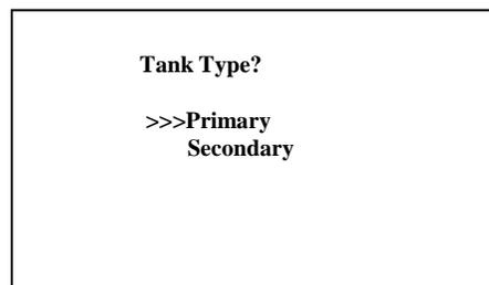
The two modes are designed for Primary clarifiers and Secondary clarifiers due to their differing Sludge characteristics.
