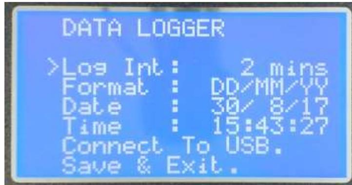
Figure 4.20 – Data Logger Set Up.
