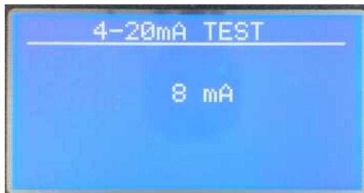
Figure 4.29 4 - 20mA test Screen.
