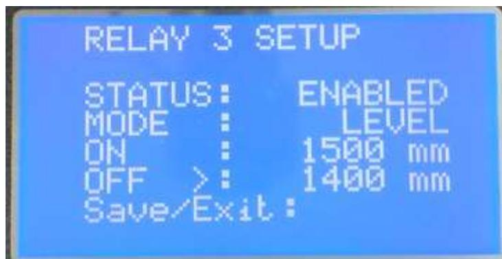
Fig 4.25 Setting Relay Parameters.
