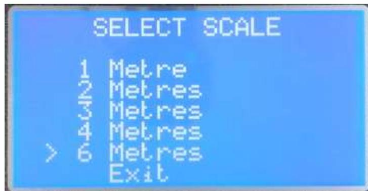
Figure 4.31 Scales for a Digisens 6 Sensor.
