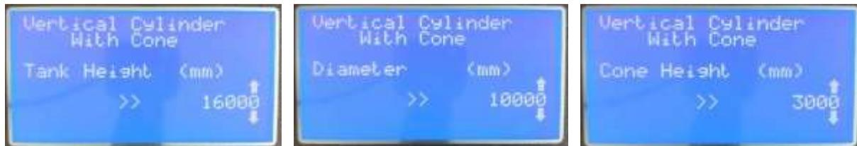
Figure 4.6a,b & c Dimension Input Screens
