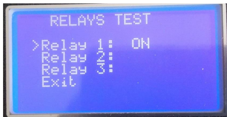
Figure 4.2 – Relays Test Screen 2
