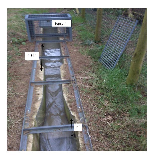
Ultrasonic sensor must be positioned a distance 4-5h where h is the maximum depth of the flume.
