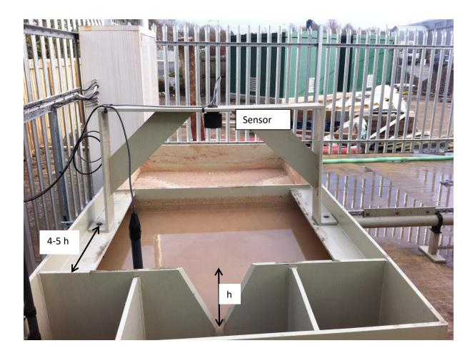
Ultrasonic sensor must be positioned a distance 4-5h where h is the maximum level of liquid above the v-notch
