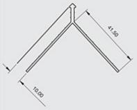
Locally manufactured from recycled plastic, Renderplas PVCu corner beads / angle beads are designed for function and speed on all external and internal rendering and plastering applications. Discreet but strong, all beading gives a perfect finish to through colour render and is equally suitable for sand and cement
