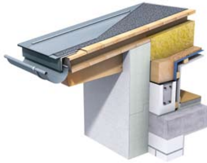
Fig. 1: Commonly used at renovations – Ventilated roof structure with insulation installed between rafters
