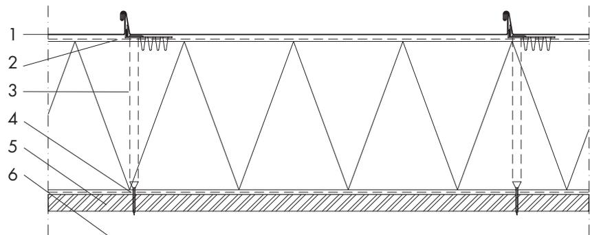
**NV 04 – ProRoofing: Non-ventilated Roof Build-up – sealed Warm Roof on Breather Membrane and Composite Panel****Characteristics**
