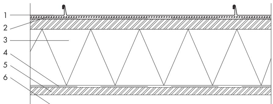
**NV 02: Non-ventilated Roof Build-up – sealed Warm Roof on structured Underlay with Warmfast Fixing**
