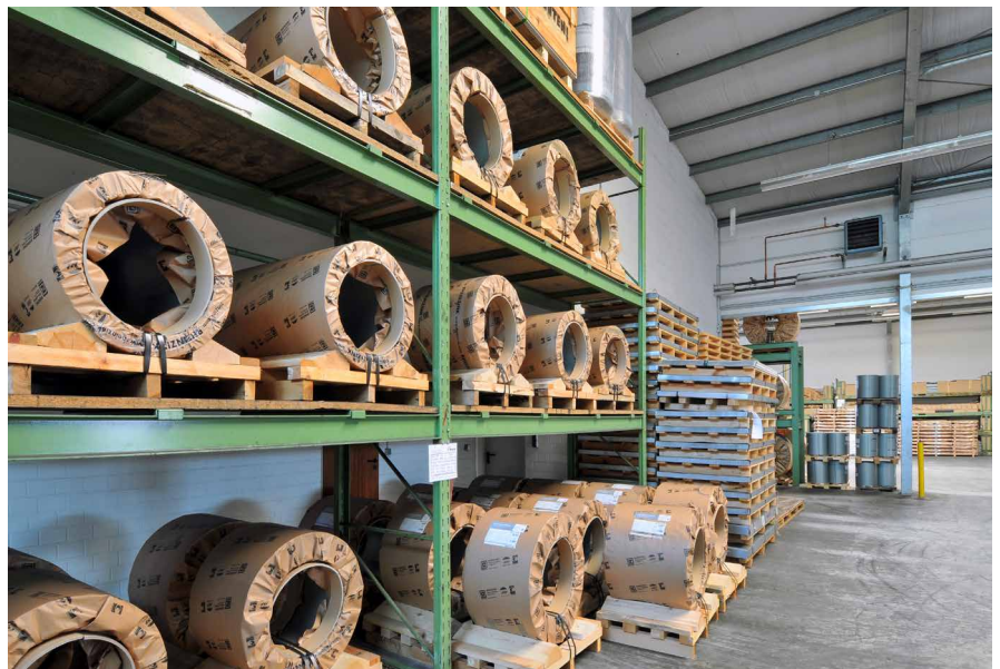
Storage of coils with wooden sleepers
