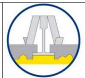
For rebated edge tiles with a deep profile pattern an increased thickness should be used. A cut piece is inserted separately into the rebate.
