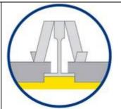
For rebated edge tiles with a flat or small surface pattern, the minimum thickness can be used. A cut piece is inserted separately into the rebate.
