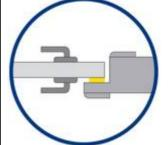
A strip of Soundseal may be fixed to the rebate of a door or window casing. Care should be taken to use the correct thickness to allow the door or window to close. For ceiling around pipes:
