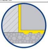
Soundseal is ideal where a partition abuts a wall and floor taking out any undulations.
