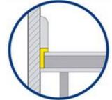
Soundseal can be fixed around perimeter walls to isolate a floating floor from the structure.
