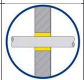
Where services pass through a wall, Soundseal is used as a gasket seal.
