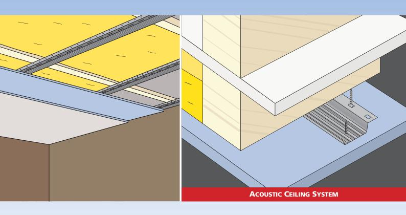
**ISOSORBA™** sound insulating ceilings systems are designed to reduce noise transmission through ceiling constructions in multiple dwellings. Not only do these systems reduce airborne sound but are also very effective in reducing impact noise too.
