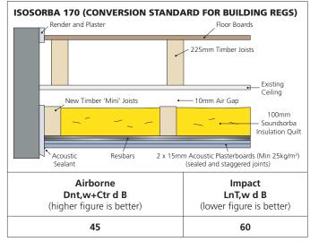
The above is typical acoustic performance based on Isosorba noise reducing ceiling systems applied to a standard existing timber joist floor with floorboards above and a plasterboard or lath and plaster ceiling.
