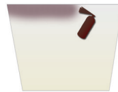
Step 3: Spray glue on backing wall surface
