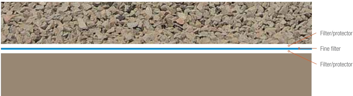
TERRAM Hydrotex composites allow pore-water pressure to dissipate whilst preventing fine clay and silt particles migrating to contaminate the ballast. In addition, an Hydrotex composite conforms to the formation profile to minimise the potential for ponding.
