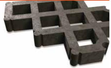
The installation was simple and quick. Each paver weighs only 9kgs – substantially lighter than concrete alternatives and they are also compliant with HSE manual handling limits – so can be easily handled by one person. The pavers (600x400x80) were butted together and the series of cells in each unit created a void area of 55%, which was filled to ensure a grass finish.
