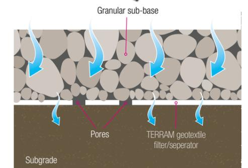
A natural filter is established adjacent to the geotextile's pores.
