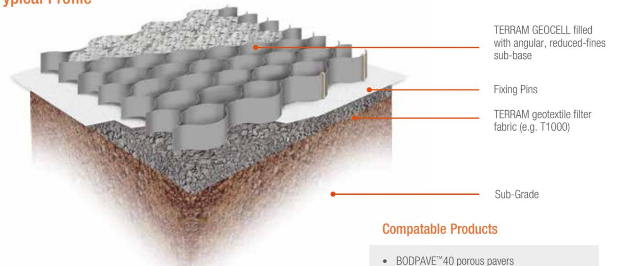
TERRAM GEOCELL filled with angular, reduced-fines sub-base
