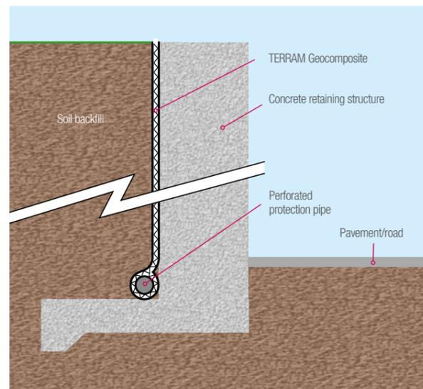
**Retaining Structures.** To maintain the stability of a retaining structure it is important to provide an efficient drainage system at the rear of a retaining structure to prevent the build up of pore pressure.
