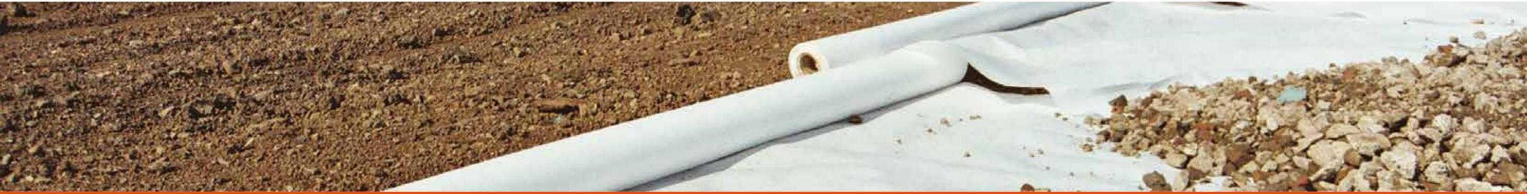
**TERRAM Standard Geotextiles prevent intermixing of sub-base and subgrade layers. This intermixing causes a loss in bearing strength, as the stone layer becomes progressively contaminated, resulting in failure in the form of deformation. This can be remedied if it's an unpaved area/road by filling the ruts but even this can be uneconomic or unacceptable if stone has to be imported over long distances at a later date.**
