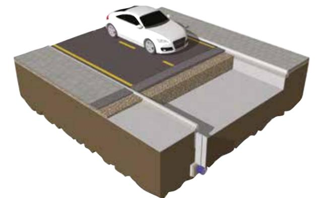
Vertical edge drains running parallel to a roadway are necessary to intercept the lateral flow of groundwater. A geocomposite fin drain saves on excavation and is quicker to install than a stone alternative.
