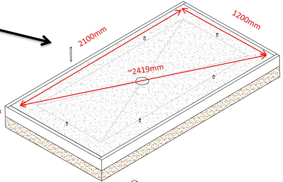
6. Install A142 steel reinforcing mesh (or similar) on 50mm plastic or steel supports or “chairs” to hold mesh vertically centred in shuttering area.
