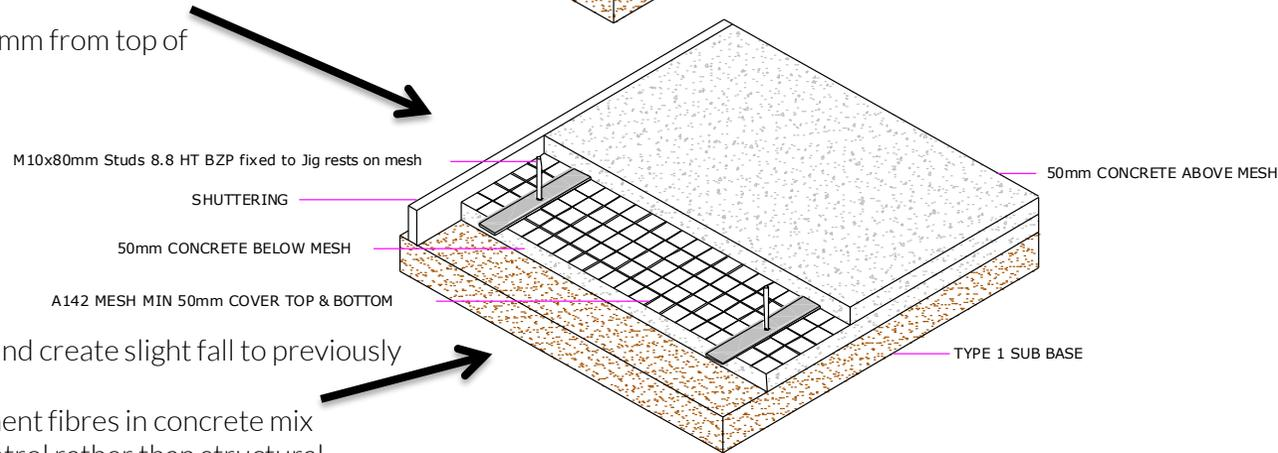
8. Pour 100mm depth concrete pad and create slight fall to previously fitted drainage inlet.
