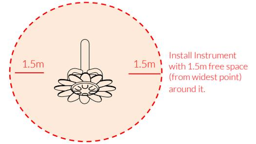
Install Instrument with 1.5m free space (from widest point) around it.
