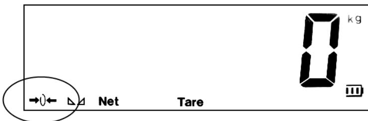
If you want to display the present weight after starting the scales (useful for container weighing), you need to change some items in the menu screen. Refer to the menu mode C07 / C08 / C09 as well as C05 to determine the internal zero position.
