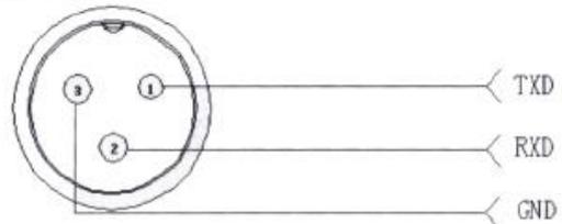
The display possesses a bidirectional RS-232 interface. This means that it is possible to control the interface with the help of query commands. Therefore, there is the possibility to send a query from your computer to the software of the scales and process the queried data afterwards.
