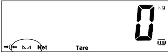
In case that the scales do not react, check the power supply of the display. If the sign for stable operation does not appear, check the subsurface and align the scales.
