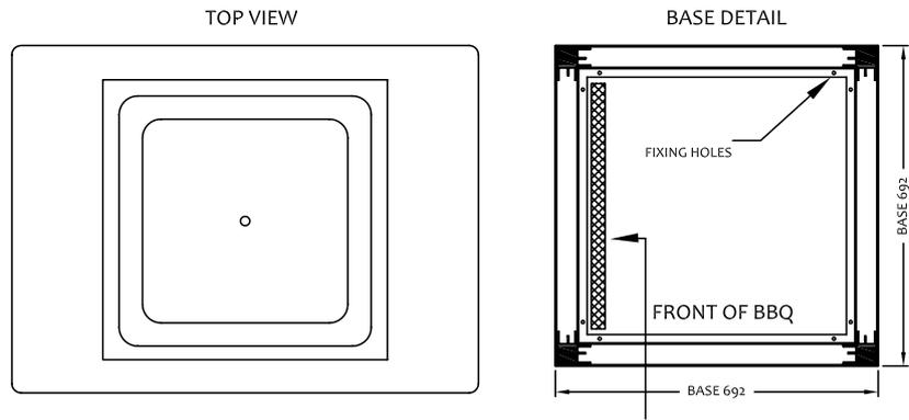
BRING UNDERGROUND SUPPLY PIPES/CABLES UP TO THE LEFT SIDE OF HOTPLATE OPENING LOOKING FROM THE FRONT AS INDICATED BY SHADED AREAS. DO NOT BRING PIPES/CABLES UP DIRECTLY UNDERNEATH HOTPLATE AND ENSURE PIPES/CABLES DO NOT RUN UNDERNEATH HOTPLATE.
