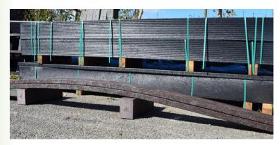
It is essential that our recycled profiles remain in pallet format i.e. stored flat and tied in bundles until the period of installation.
