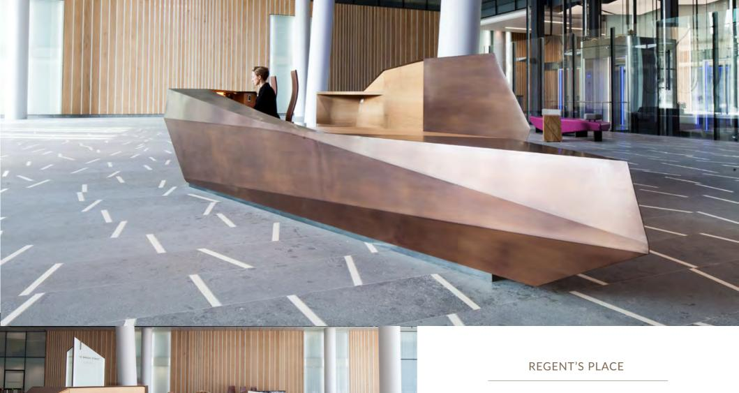
Modelled first on CAD and then deconstructed into individual components to be programmed for the CNC machine, the enormous, multiangled reception desks are clad in guilding metal, expertly bent, welded and polished for a seamless finish.
