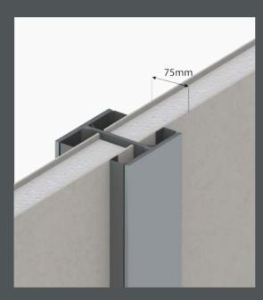
Guardian Wall<sup>™</sup> Extended design life with HDG UB posts. Wall Heights: Up to 9000mm Panel Span/Post Centres: 2040mm - 3040mm Post Dimensions: Dependant on application and region
