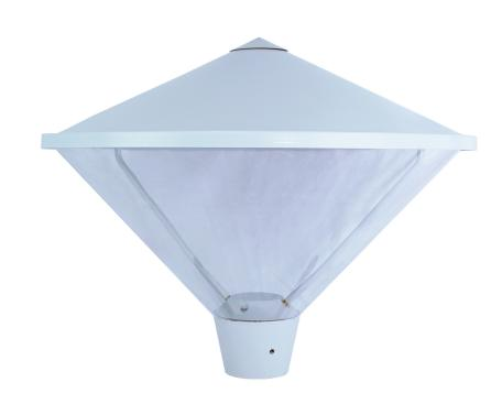
A stylish IP66 rated post top amenity lantern with aluminium cast body and spigot adaptor. UV stabilised polycarbonate cover rated IP66 and IK10. Design to suit any modern environment with superior photometric performance. Best suited to campus environments and regeneration schemes the Chelsea offers contemporary design aesthetics without compromising performance. Manufactured from the highest quality materials all sourced in Britain.
