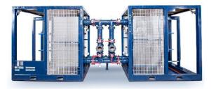
The OSSO single and dual high volume mud coolers incorporates either one or two plate heat exchangers designed specifically for drilling mud and in accordance with PED/ASME codes and standards. They have inlet /outlet pressure and temperature gauges, and the dual mud cooler can be operated as an individual unit, or in series.
