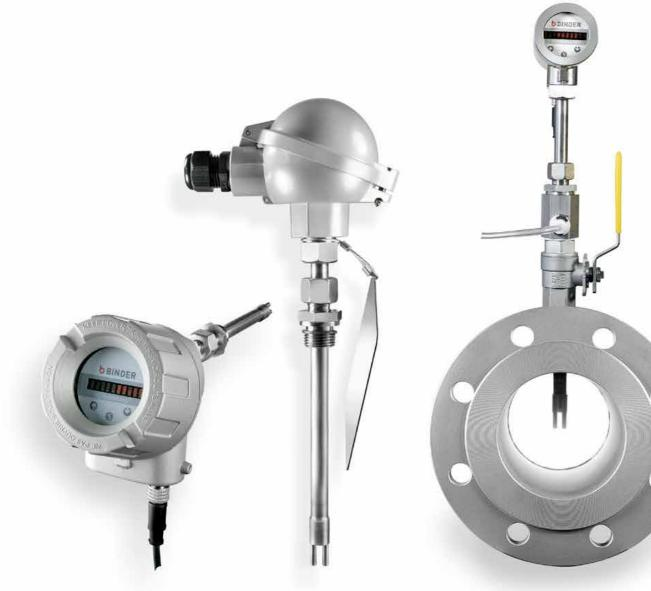
Each flow meter is tested prior to shipment and calibrated at our CAMASS<sup>®</sup> Calibration Lab under actual operating conditions (piping layout, gas composition, pipe diameter, flow direction...). The sensor uses the thermal dispersion principle and directly measures the gas mass or volumetric flow at standard pressure and standard temperature (according to DIN 1343: 0 °C, 1,01325 bar, 0 % rel. humidity) in dry gases. It consists of a heated
