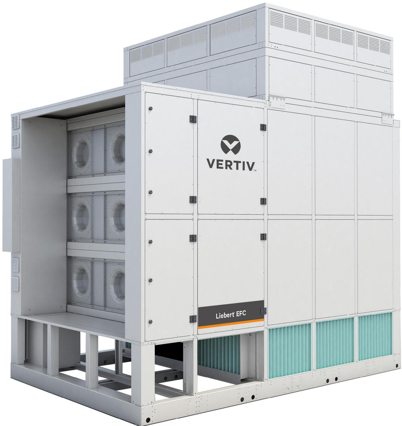
The evaporative system has a dedicated internal pump that provides the water needed. Water is sprayed through special nozzles onto the heat exchanger and evaporates, thus humidifying and cooling the air.
