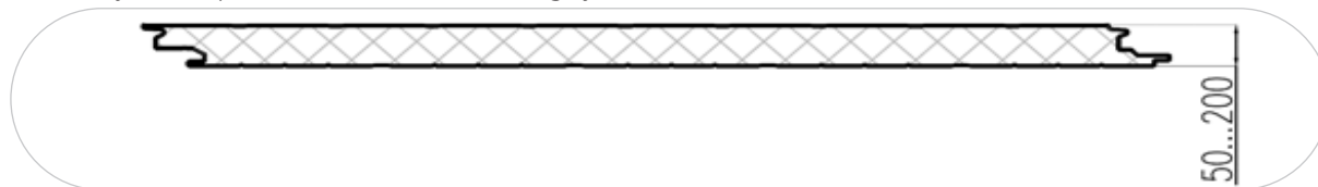
Figure 20. Geometry of wall panels with Secret Fix locking system (PWT SF)
