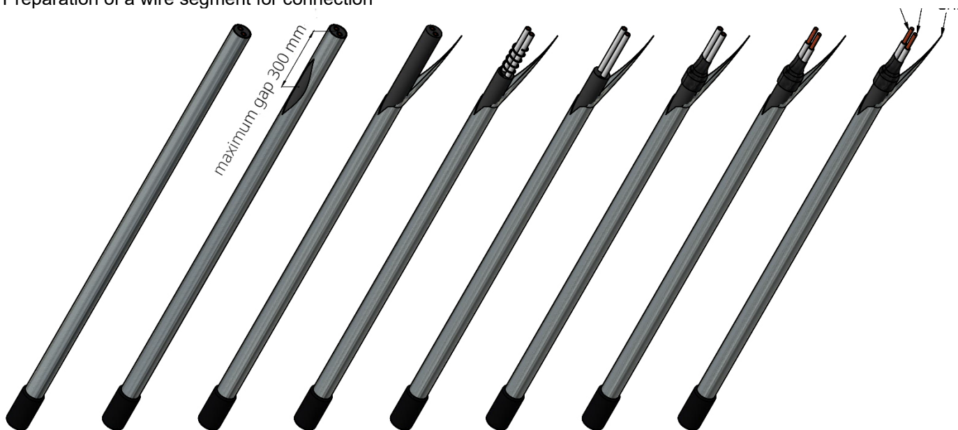
Figure 15. Preparation of a wire segment for connection
