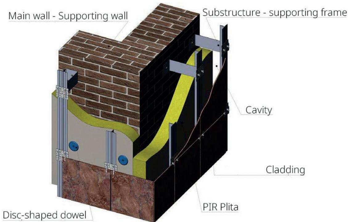
The attaching of PIR Plita® to the wall should be done using disc dowels. The insulation boarding is fixed to the brackets and then mounted. After that, the cladding is attached.
