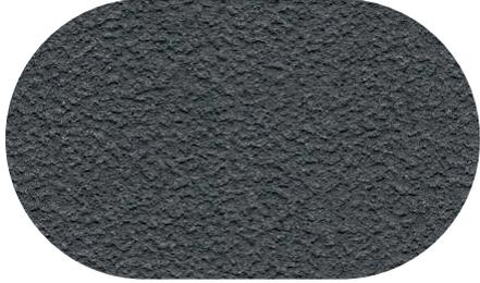
Fiberglass base with additional graphite and flame retardant coating. For use on the external cladding of walls and facades. Density 630–700 g/m<sup>2</sup>, thickness 1.10 mm (± 15%)
