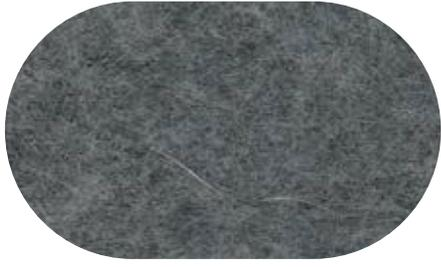
Bitumen coated fiberglass base with polypropylene. Mainly used on the construction of pitched roofs and flat roofs. Density 330–370 g/m<sup>2</sup>, thickness 0.72 mm (± 15%)
