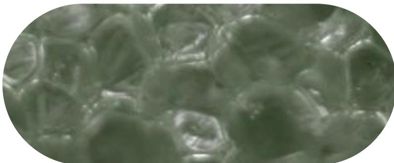
Polyisocyanurate PIR foam is very popular due to its high resistance to fire. Its defining feature in this regard is its ability to charr during combustion or when it is exposed to flame, due its "porous" carbon matrix. This matrix protects the inner layers and prevents them from burning. In addition, due to the structure of the matrix, significantly less heat is generated than with other foams which burn completely. The operating temperature of PIR Plita® is up to 120 °C.
