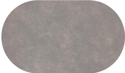
Fiberglass base with breathable waterproofing membrane. For use on roofing of a wooden truss system. Density 190 (± 5%) g/m<sup>2</sup>, thickness 0.9 mm (±15%).
