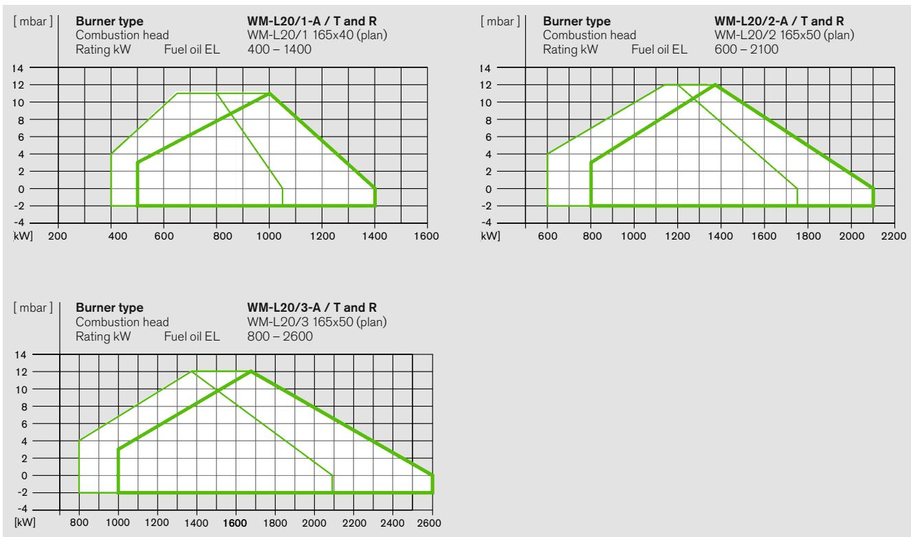
**Fuel oil EL: Capacity with combustion head**
