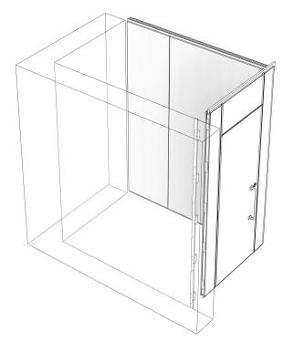
Wall Pilasters are grooved top & bottom to receive front in-fills and is haunched out to take softwood fillets to create a secure connection to the wall. Black compact laminate flash gap spacer is fixed to the side wall.
