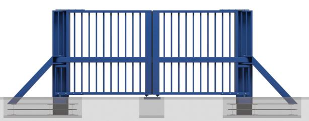
**Applications:** High Security sites which require equipment that meets a higher level of PAS 68 specification and have a lack of runback area for sliding gate.
