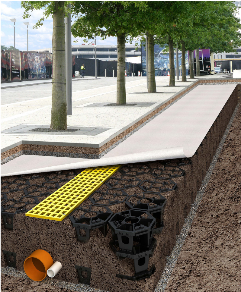
Load bearing deck for spanning shared utility trench.
