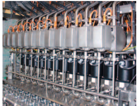
Dosimass flowmeters operating in a 12-lane line filler
