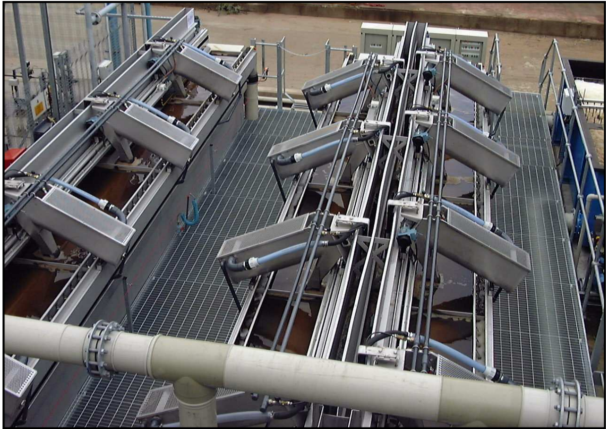
Top view of filters showing sand washers
