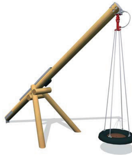
Main beam Ø 24 cm, feet Ø 18 cm, robinia Ø 24-28 cm
